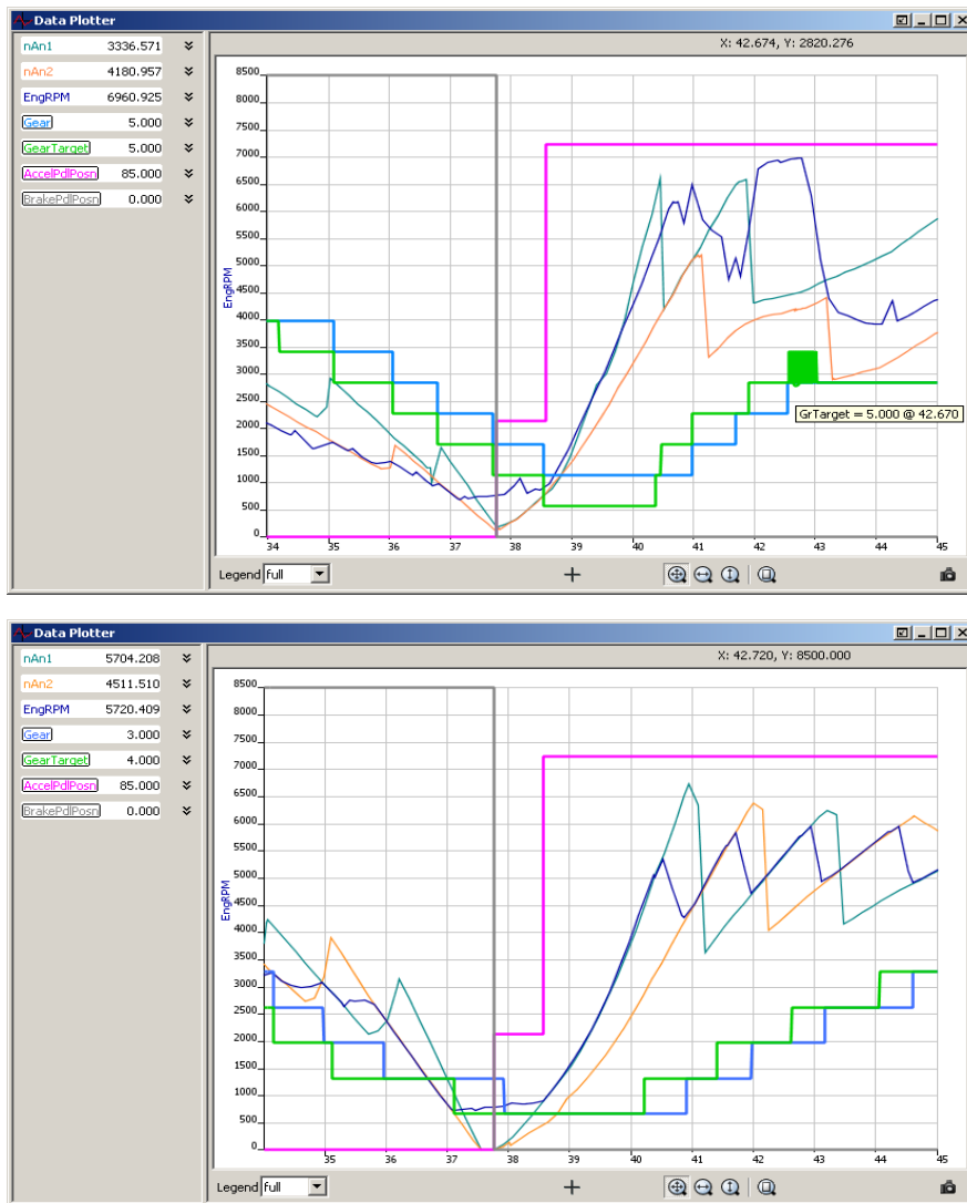
Fig 8: Oscillating target gear (green) before and after a bug fix
